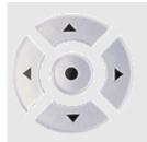
Navigation Buttons: These arrows keys serve as up/down/left/right button when used in the GXV3140's menus. The middle button is used as the submit/select button.
