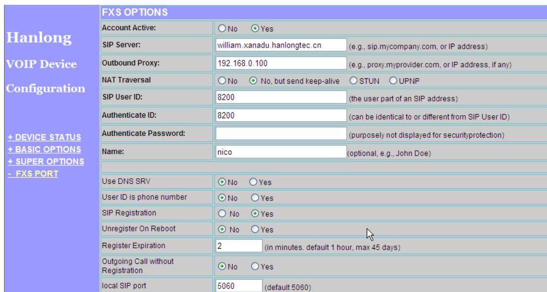
The screenshot shows the 'FXS OPTIONS' configuration page. On the left is a navigation menu with 'Hanlong VOIP Device Configuration' and expandable sections for '+ DEVICE STATUS', '+ BASIC OPTIONS', '+ SUPER OPTIONS', and '- FXS PORT'. The main content area contains the following fields:
