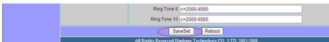
The Unicorn 3001 will then display the following screen to confirm that the changes have been saved. Please allow 5 to 10 seconds before rebooting the device.
