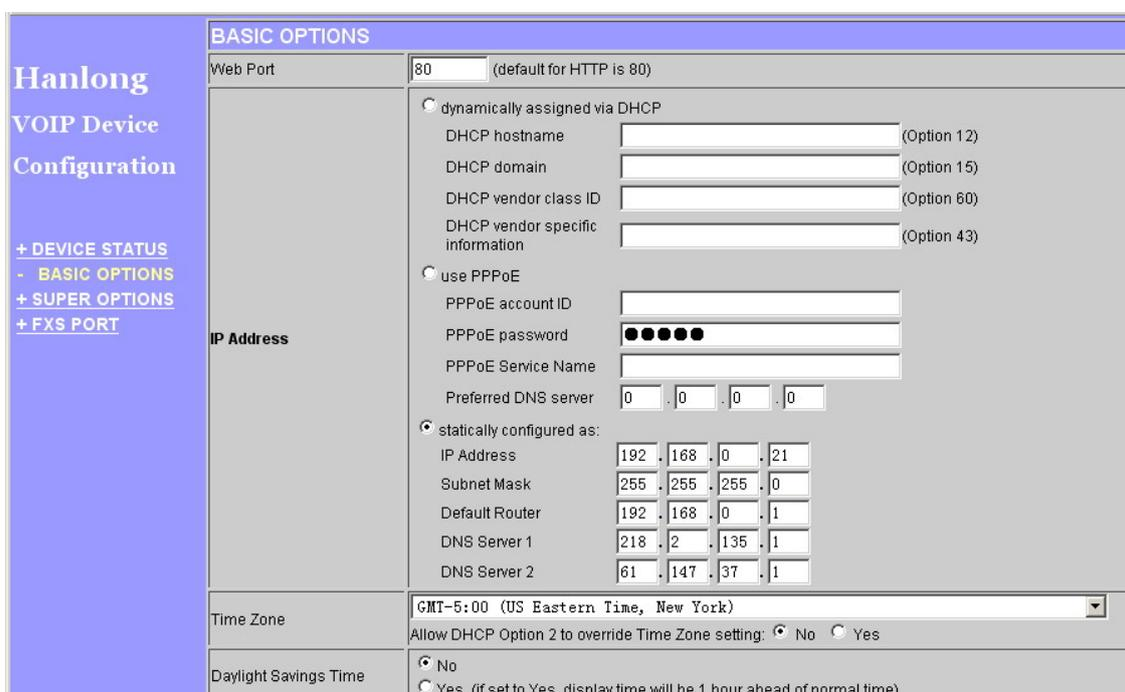
The screenshot shows the 'BASIC OPTIONS' configuration page. On the left is a navigation menu with 'Hanlong VOIP Device Configuration' and links for '+ DEVICE STATUS', '- BASIC OPTIONS', '+ SUPER OPTIONS', and '+ FXS PORT'. The main content area is titled 'BASIC OPTIONS' and includes the following settings:
